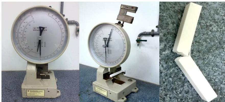
**Figure 8: Overview of Impact or Charpy Test**
